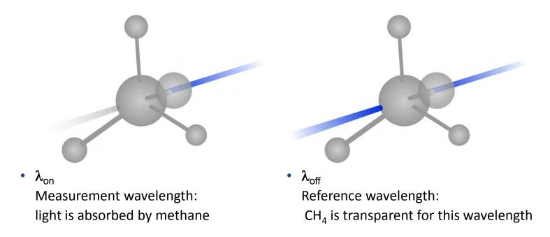
A difference in the backscatter signal indicates the presence of Methane
