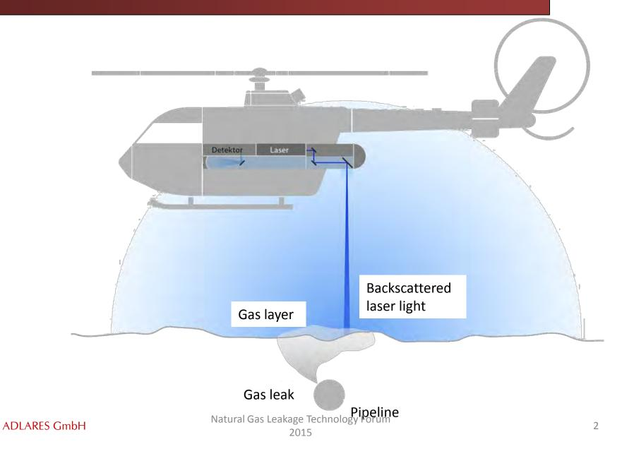
System emits laser pulses with two different wavelengths:
